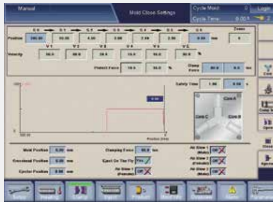
Mold protection function with 2 steps in standard.
