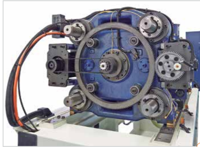
Image 1 The redesigned 5-point-toggle-system increases the platen intensity, reduces platen inertia and joint stress. This delivers an optimized speed curve and reduced dry cycle times.
